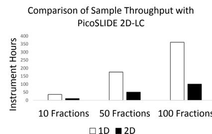
Fig 5. Instrument time needed to run a multi-dimensional fractionation method can be reduced by 70% or more depending on gradient lengths, data based on 1hr load/elute cycles.
