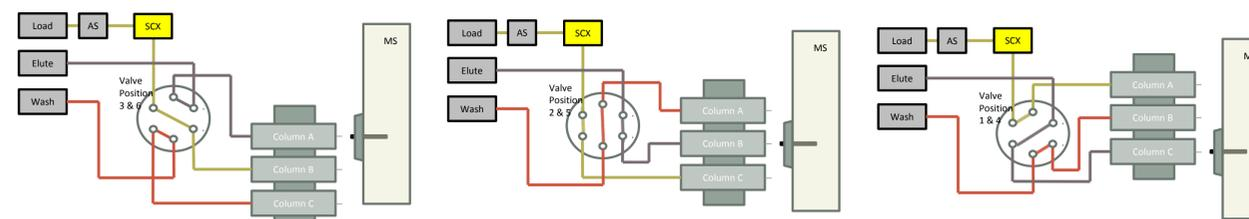
Fig 3. Schematic depicting linear isolated Load/Elute/Wash pump flow paths and valve switching mechanism when each column is in position and eluting peptides.
