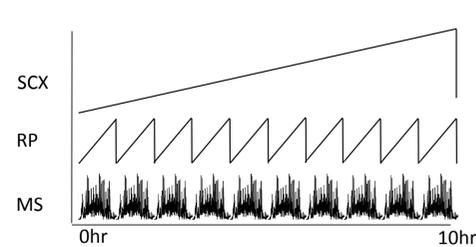
Fig 4. Diagram detailing the timing of the salt gradient, reverse phase gradients and the acquisition of the MS data.
