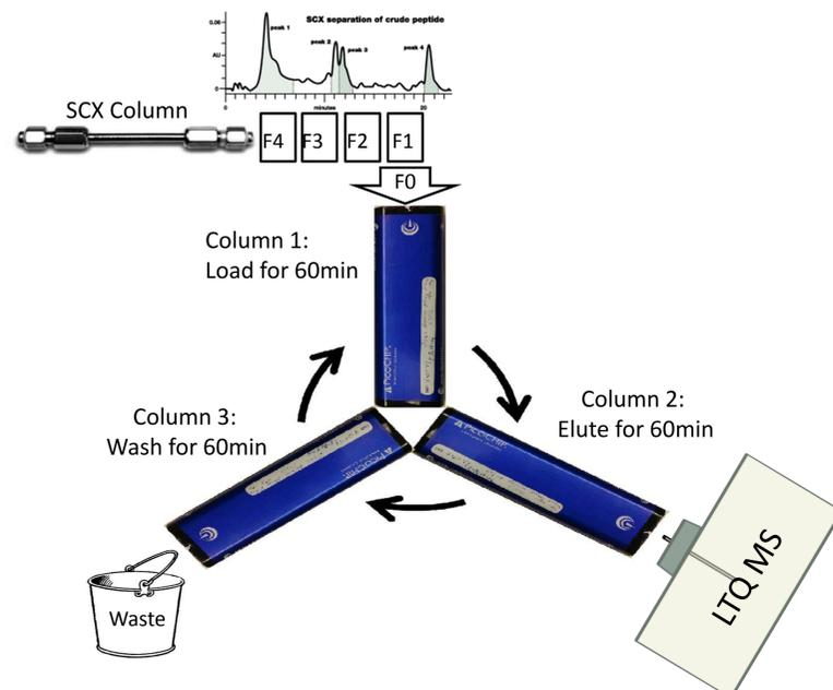
Fig 1. Diagram showing the simultaneous on-line loading of SCX separated peptides, elution via reverse phase, and washing/re-equilibrating of three PicoCHIP nanospray columns.
